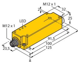
2-channel isolating switching amplifier with M12x1 males, for peripheral use, IP67, zones 2/22, input circuits II(1) Ex ia, PNP transistor output NO
