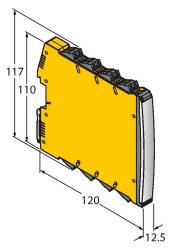
Isolating switching amplifier, 2-channel; SIL2 acc. to IEC 61508; Ex-proof version; 2 transistor outputs; input Namur signal; ON/OFF switchable monitoring of wire-break and short-circuit; toggle between NO/NC mode; signal doubling; removable screw terminals; 12.5 mm wide; 24 VDC power supply
