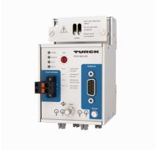
The FOC12... fiber optic media converter converts RS485-IS signals, e.g. from PROFIBUS-DP or Modbus RTU, on copper cables into optical signals and vice versa. Intrinsically safe bus signals from zone 1 can thus be transmitted intrinsically safe, potential-free and interference-free over long distances.
