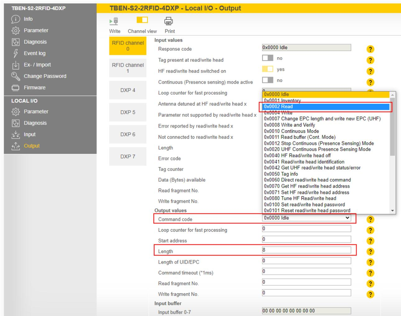
Fig. 85: Setting the read command in the web server
