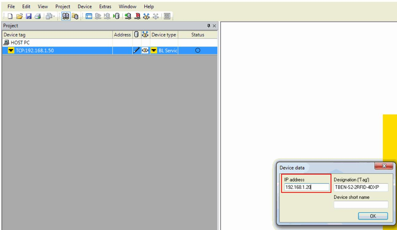
Fig. 93: Entering the IP address
