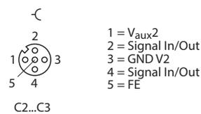
Fig. 26: Connections for digital sensors and actuators — pin assignment
