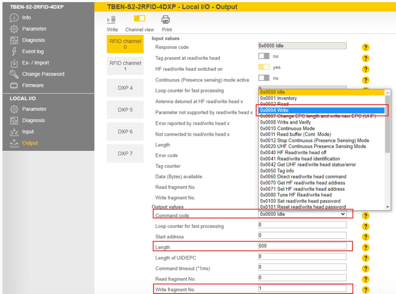
Fig. 132: Fragmentation — executing a write command
