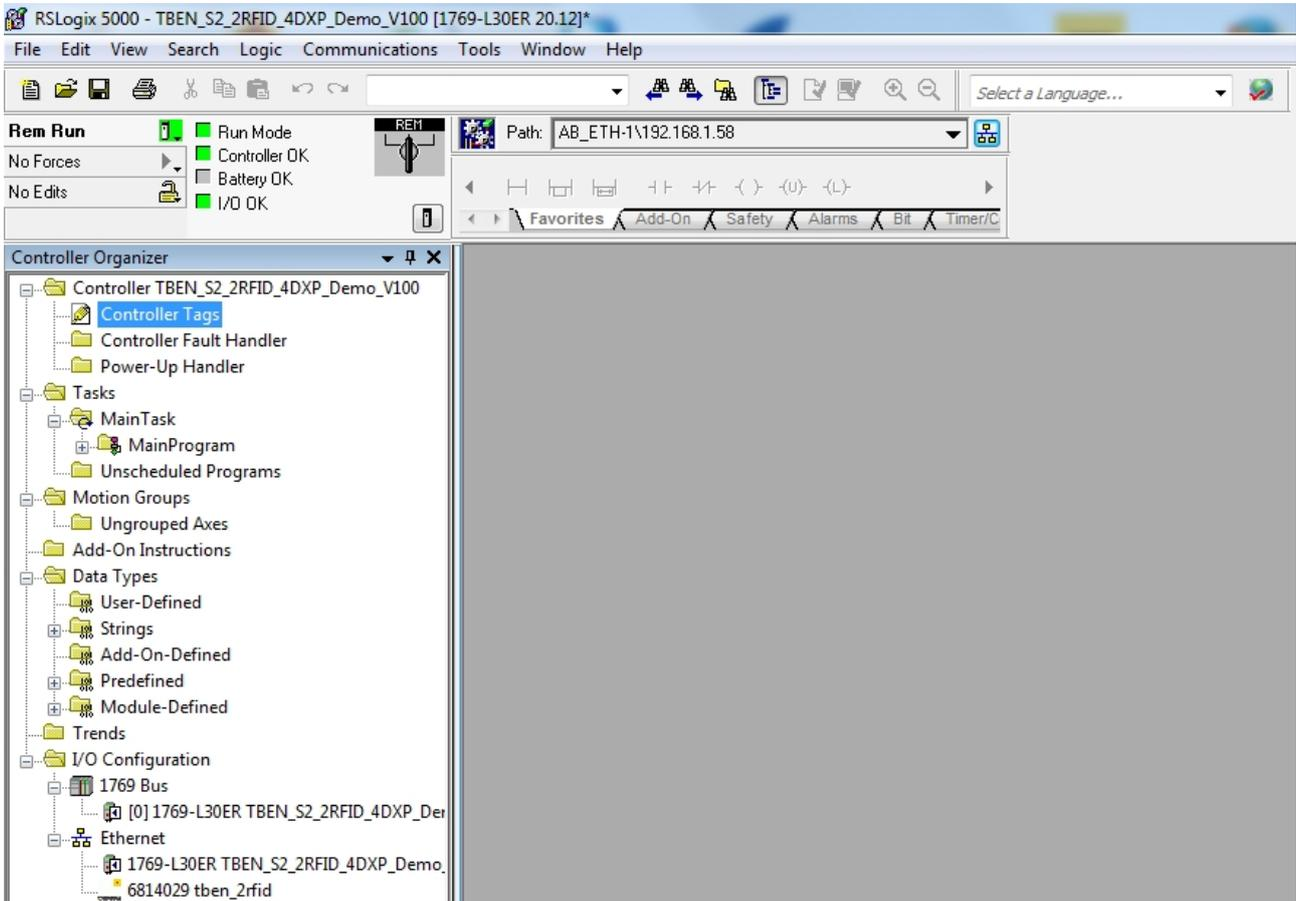
Fig. 60: Controller tags in the project tree
