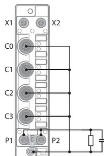
Fig. 8: Equivalent circuit, shielding concept
