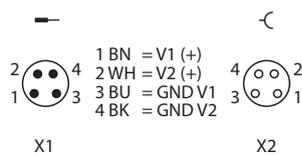
Fig. 17: Pin assignment of the power supply connections
