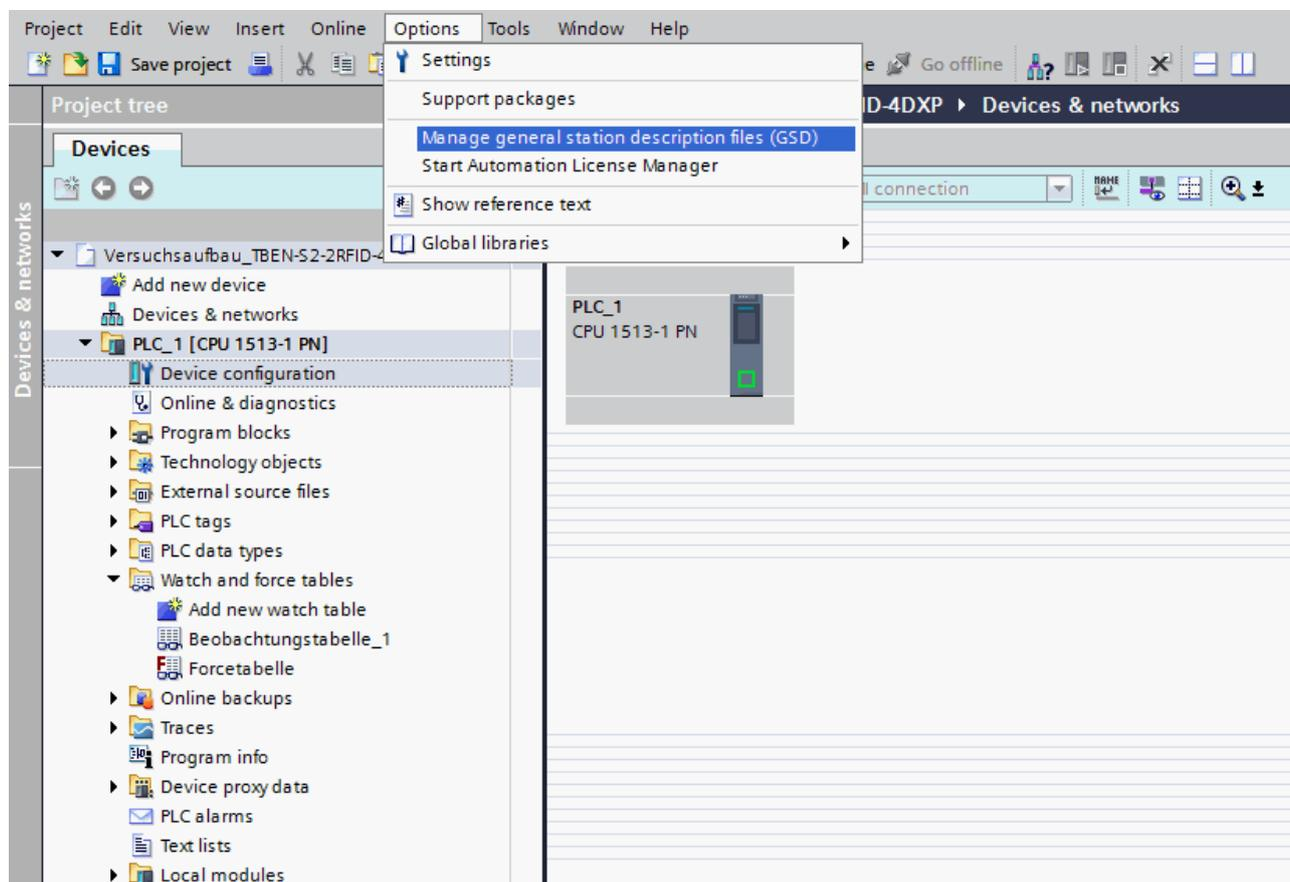
Fig. 66: Include the GSDML file
