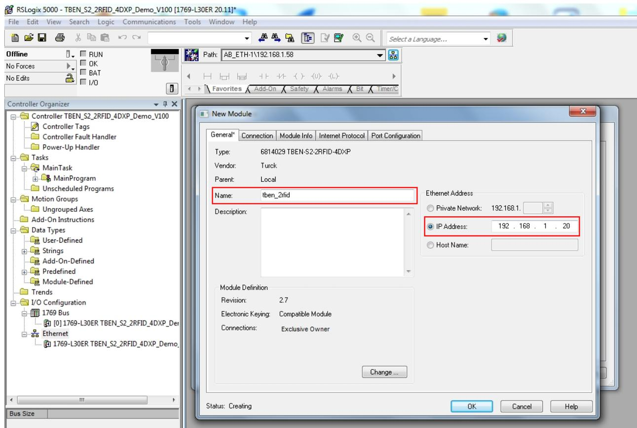
Fig. 53: Setting the module name and IP address
