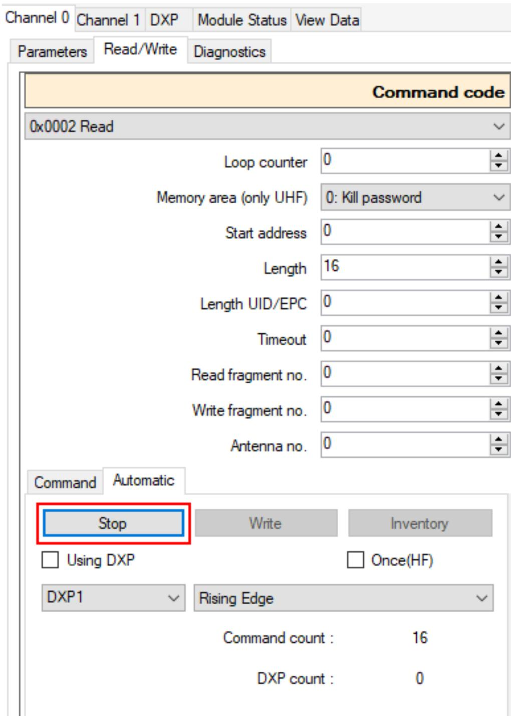
Fig. 115: Automatic mode — stop read command
