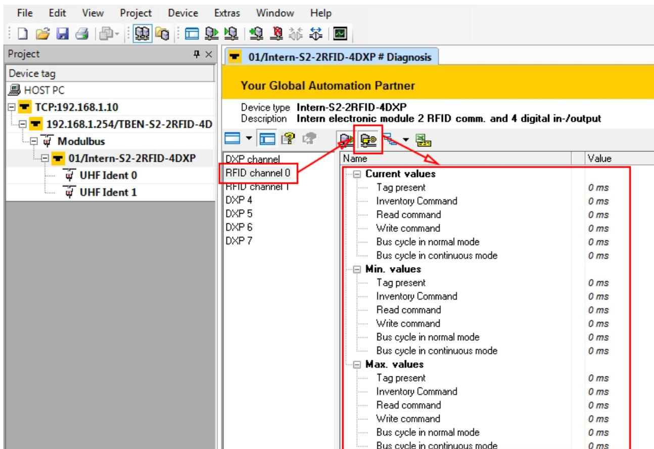
Fig. 155: Time measurement in the DTM
