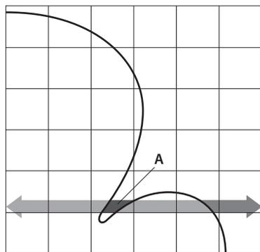
Fig. 73: Detection range of a read/write head
