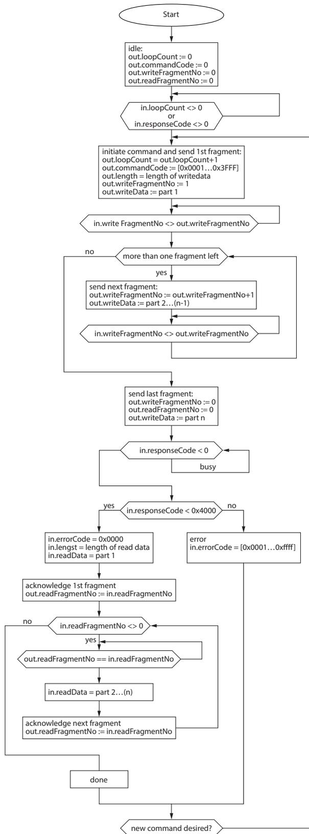
Fig. 177: Flow chart for command processing with fragmentation
