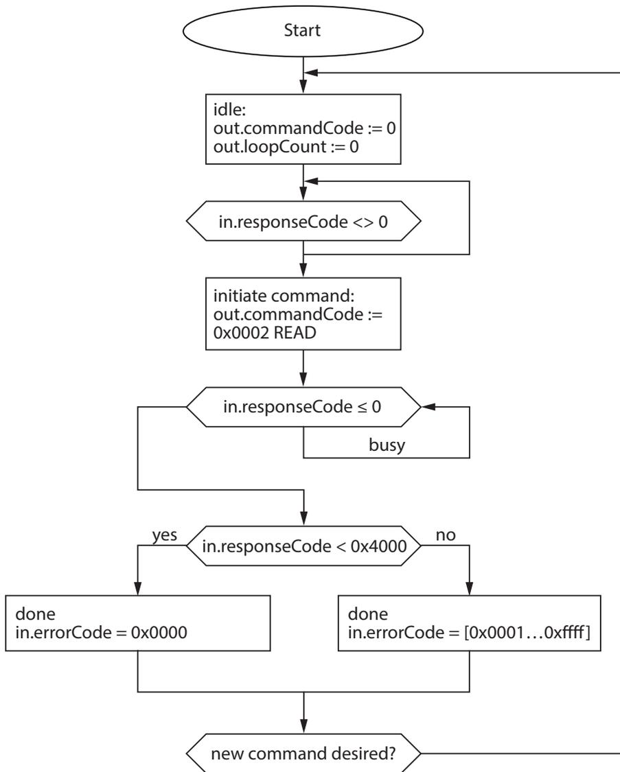
Fig. 175: Flow chart for command processing
