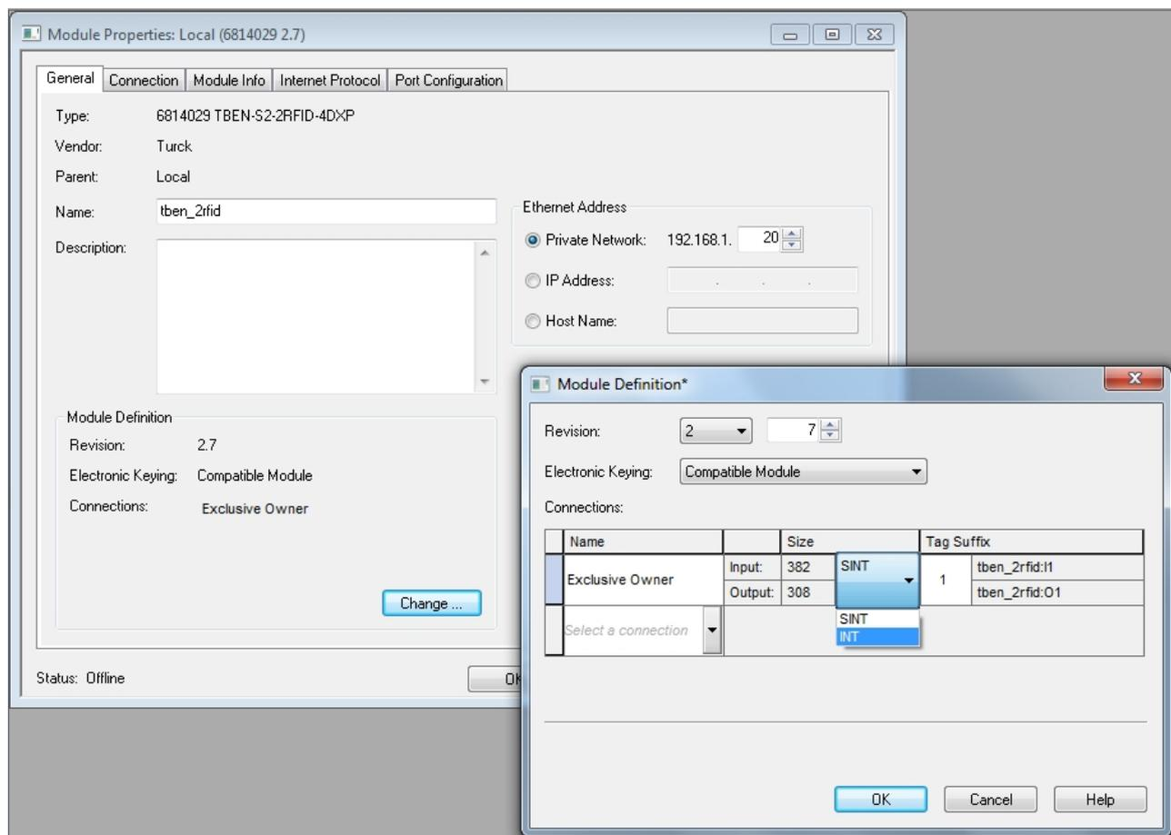
Fig. 54: Selecting an integer as a format for the input data and output data
