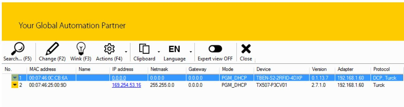
Fig. 30: Turck Service Tool — selecting the device to be addressed
