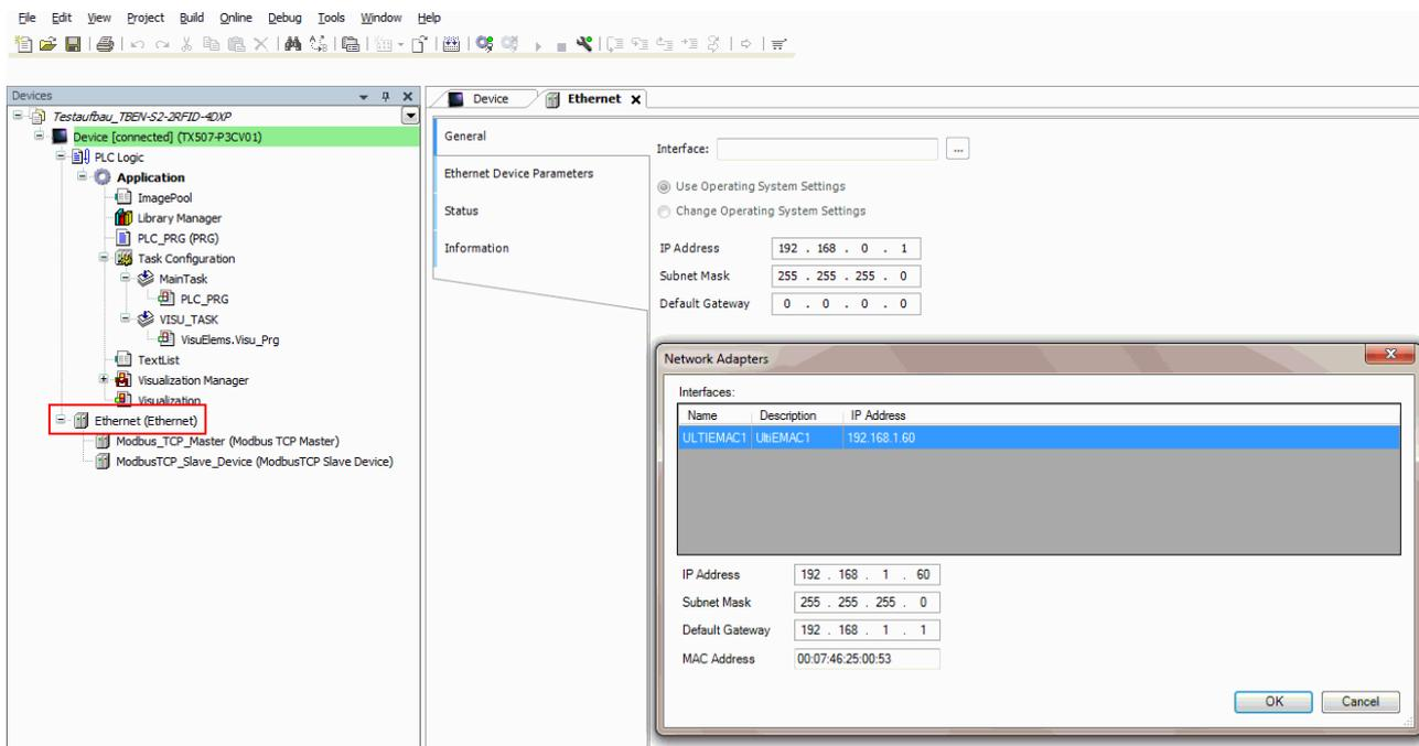
Fig. 42: Modbus slave — entering the IP address (here: 192.268.1.61)
