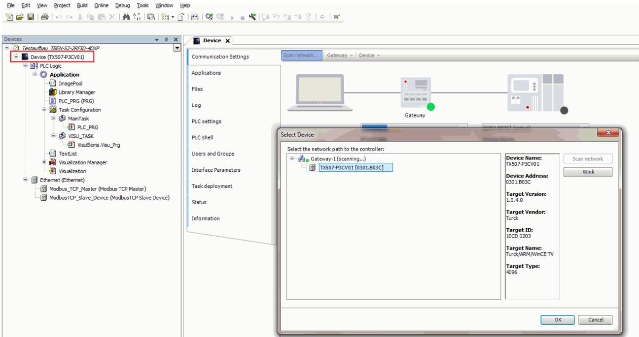
Fig. 40: Setting up a network interface to the Modbus master
