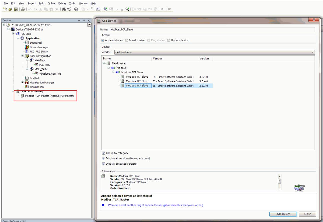
Fig. 38: Adding a Modbus slave
