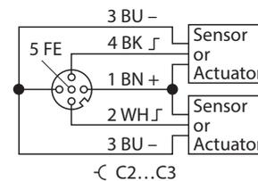
Fig. 27: Connections for digital sensors and actuators — wiring diagram
