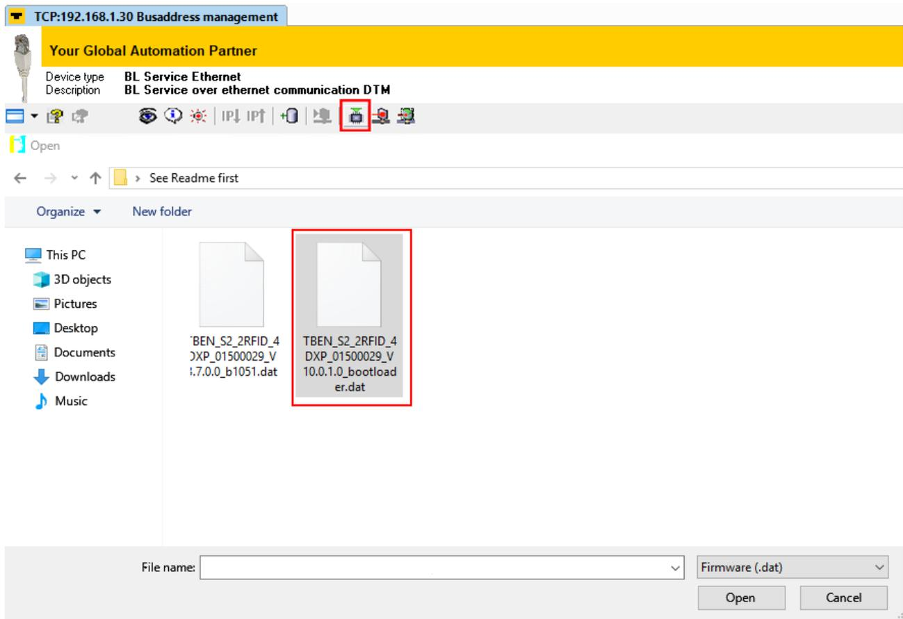
Fig. 172: Selecting the bootloader
