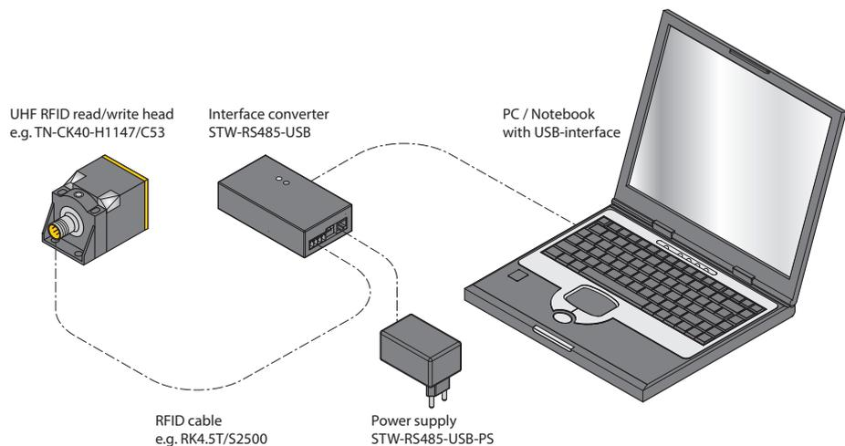
Fig. 75: Connecting the read/write head to a PC via the interface converter
