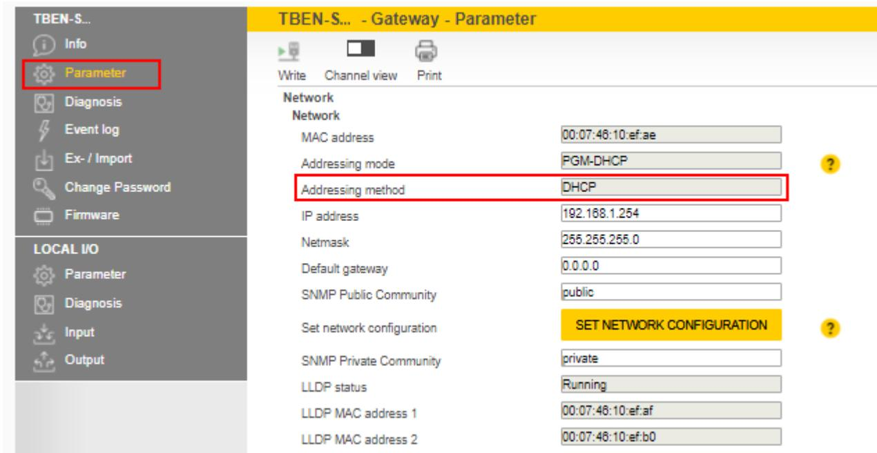
Fig. 32: Displaying the set addressing method
