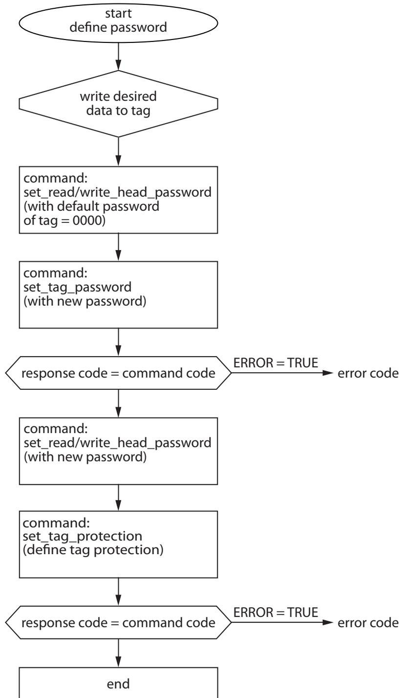
Fig. 180: programming tags with a password
