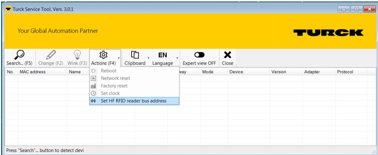
Fig. 76: Selecting a function — set HF RFID reader bus address
