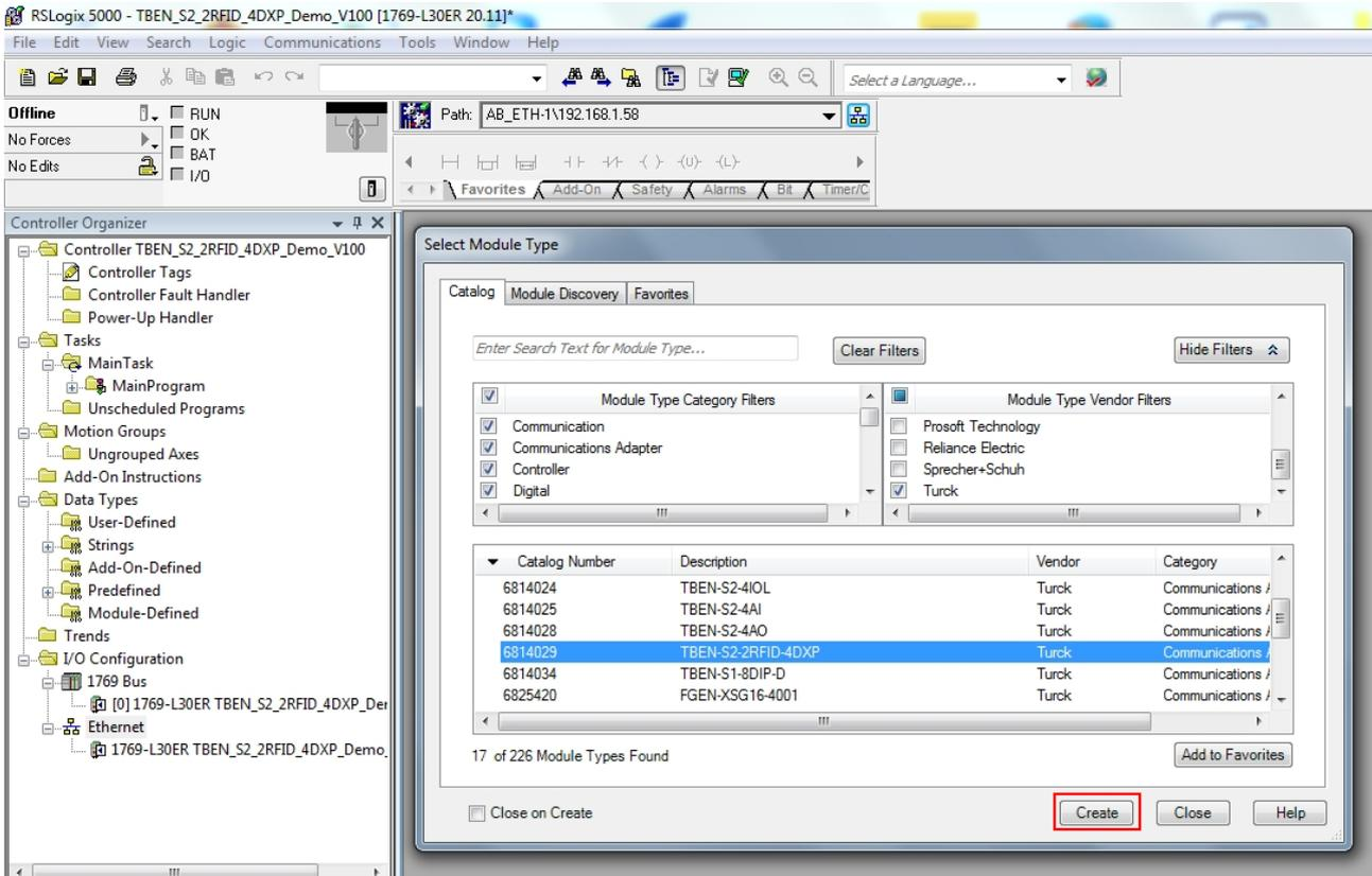
Fig. 52: Selecting an EDS file for TBEN-S2-2RFID-4DXP
