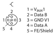
Fig. 19: RS485 — pin assignment of the read/write device connections
