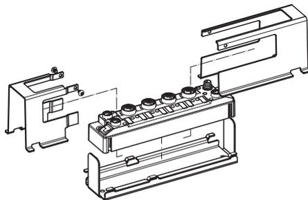
Fig. 3: Installing the device in the TB-SG-S protective housing
