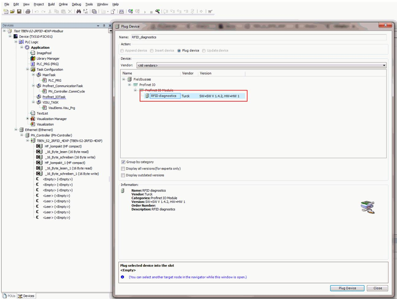
Fig. 152: Selecting RFID diagnostics
