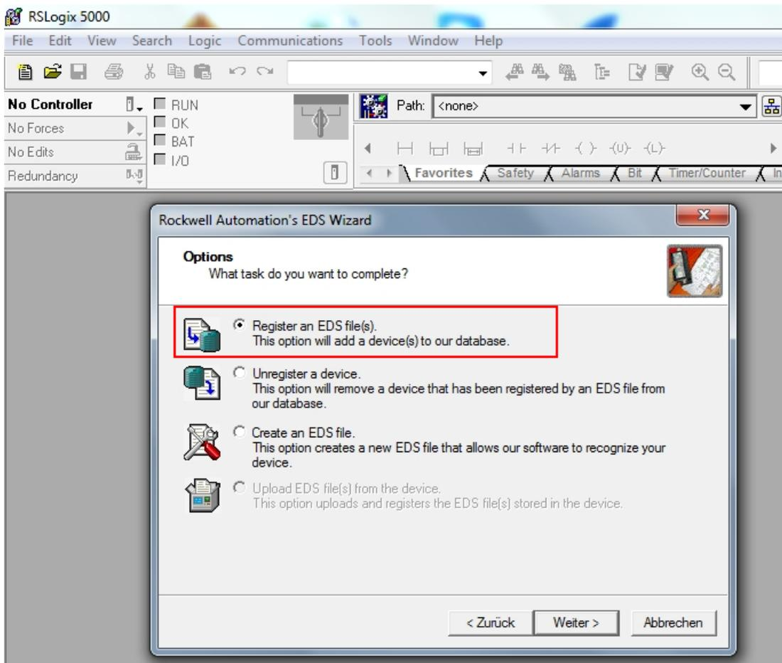
Fig. 49: Option selection — registering an EDS file(s)
