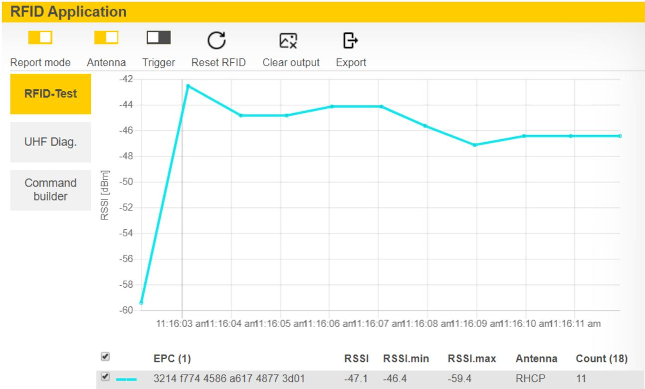
Fig. 123: Example of RFID test: Detection a tag with the received RSSI values over time and the number of read operations
