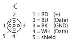
Fig. 22: .../S2503 connection cables — pin assignment of the read/write device connections
