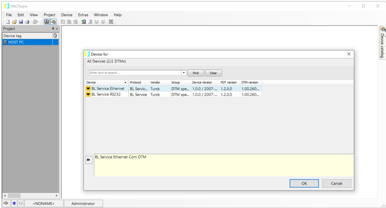
Fig. 168: Selecting the Ethernet interface
