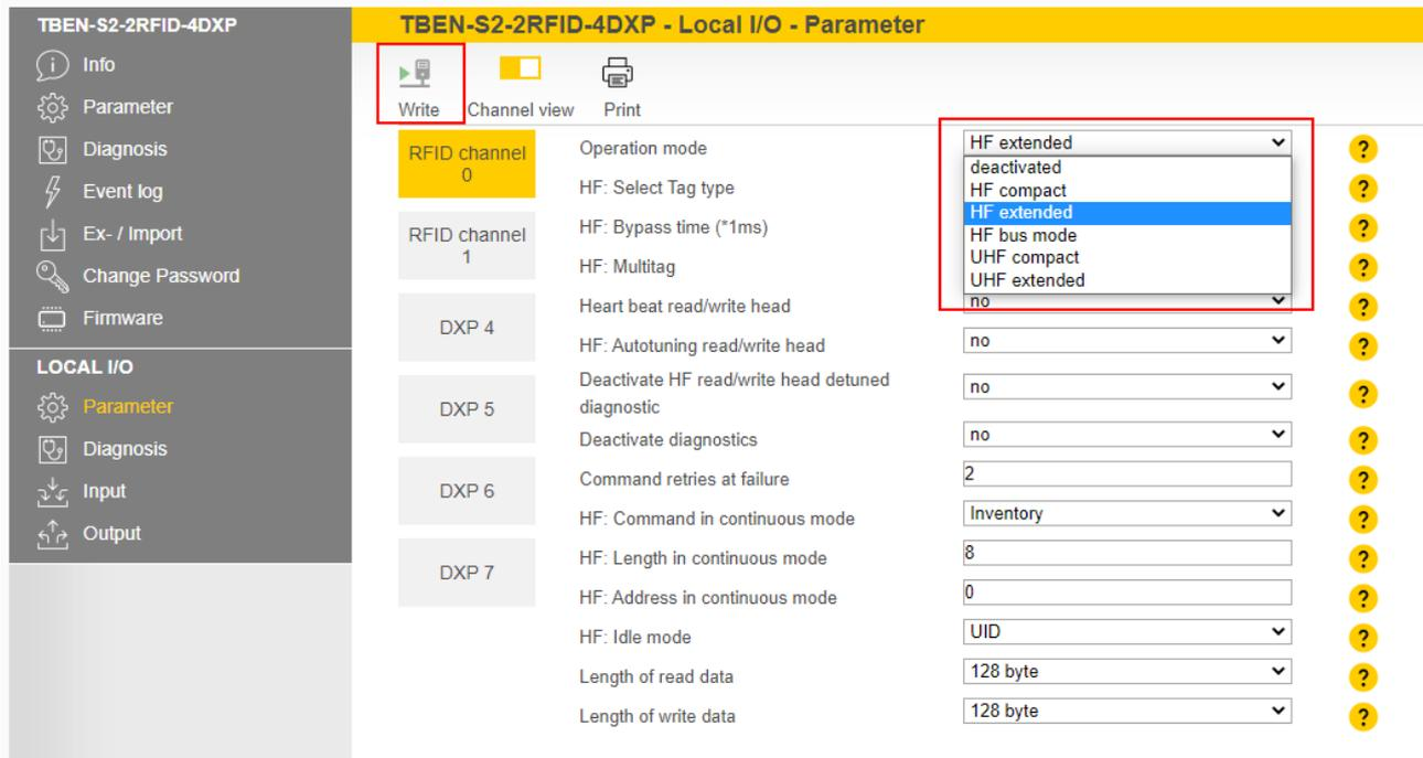
Fig. 131: Fragmentation — selecting the operating mode
