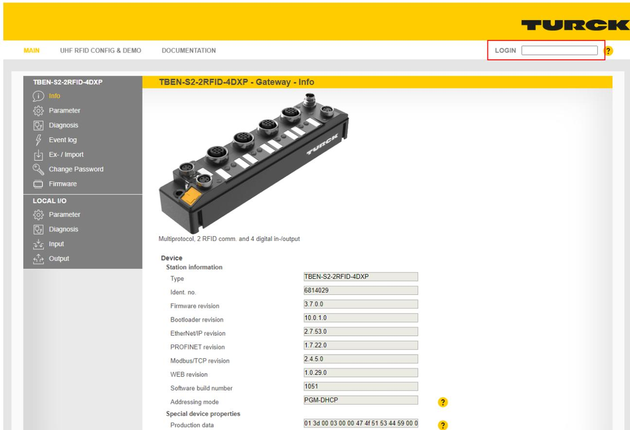
Fig. 80: Login field on the home page of the web server (marked in red)
