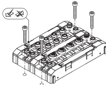
Fig. 6: Attaching the device to the mounting plate
