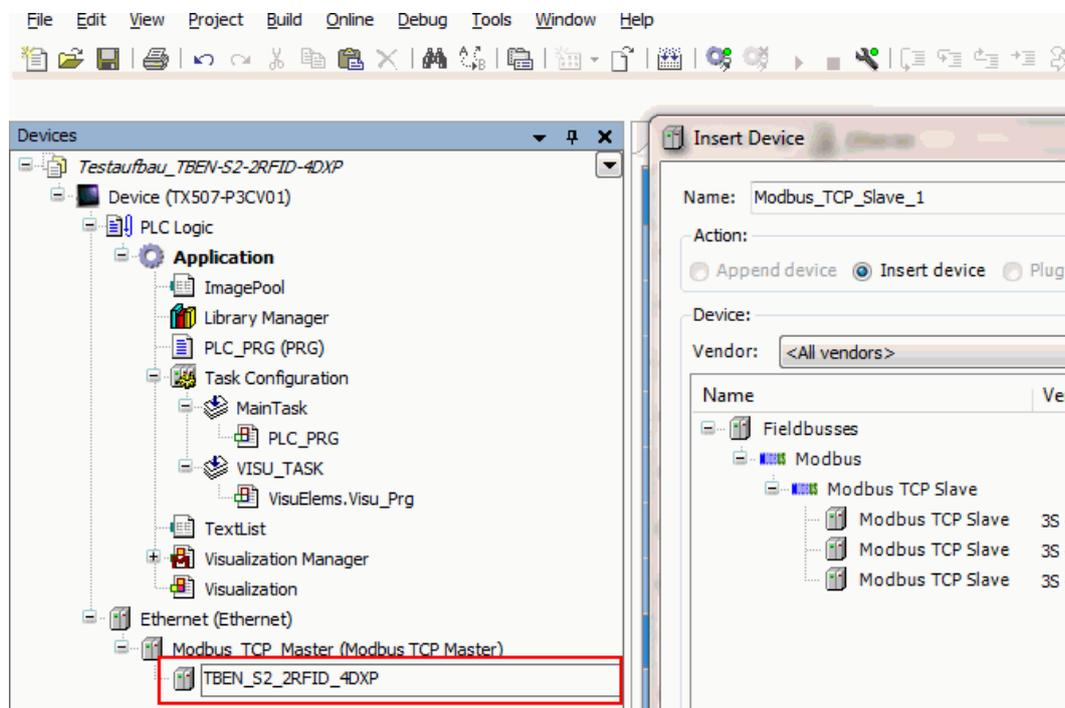
Fig. 39: Assigning a device name (here: TBEN-S2-2RFID\_4DXP)
