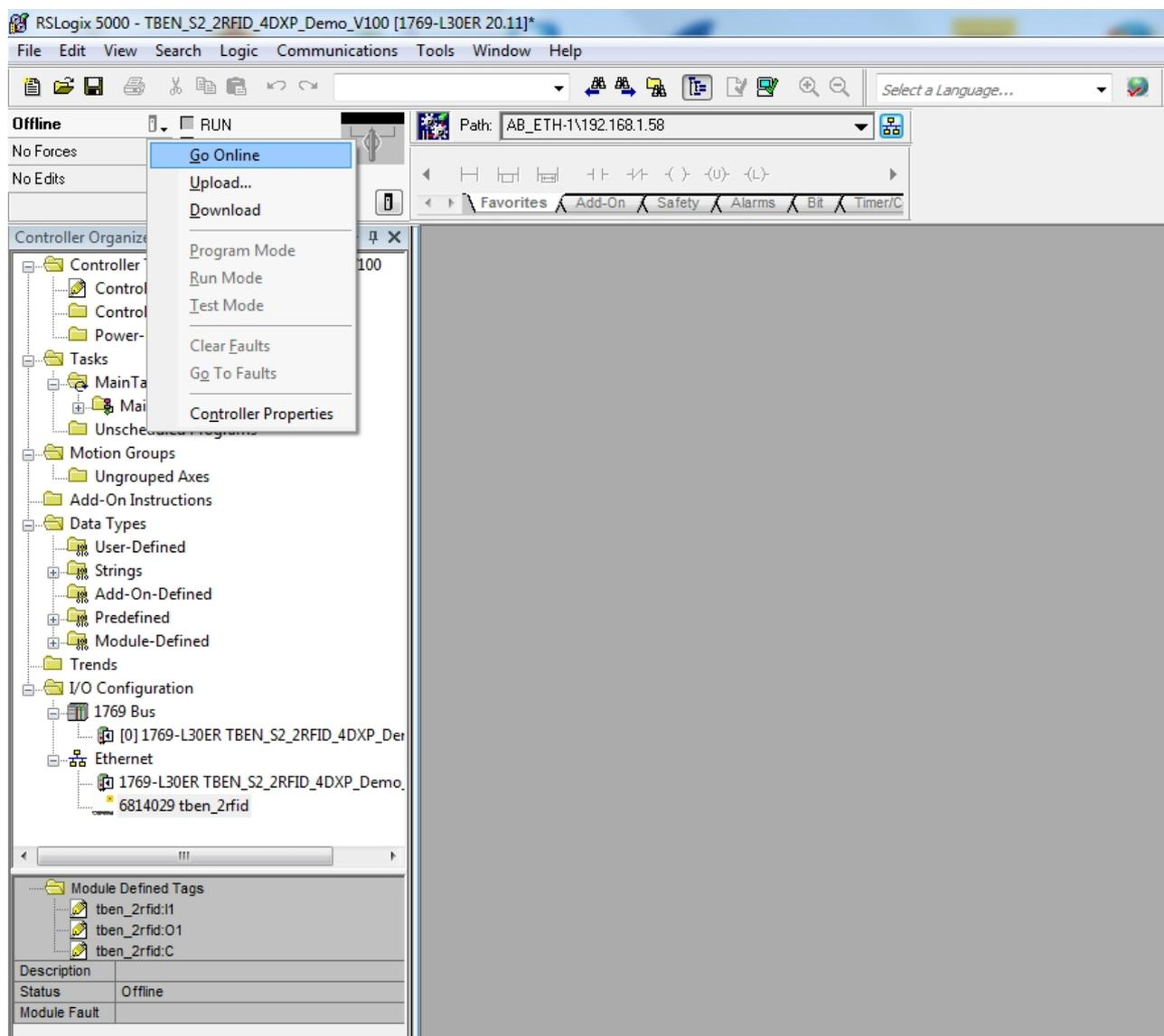
Fig. 58: Connecting the device online
