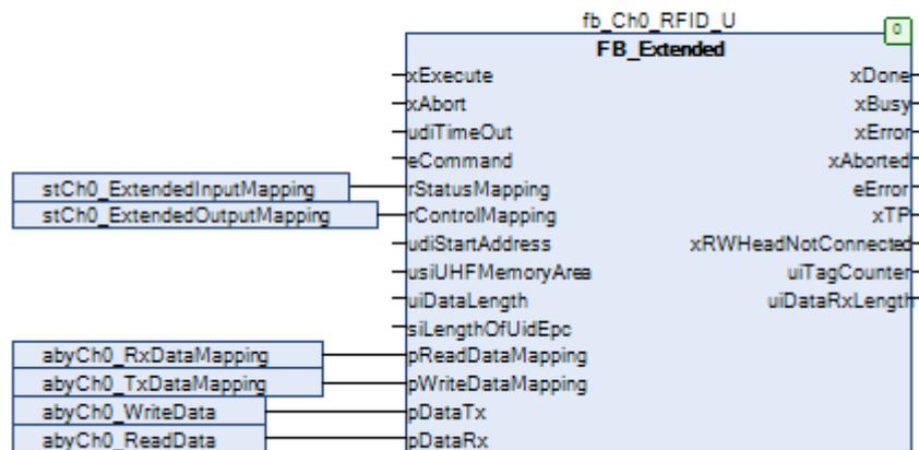
Fig. 146: FB\_Extended function block — overview of inputs and outputs
