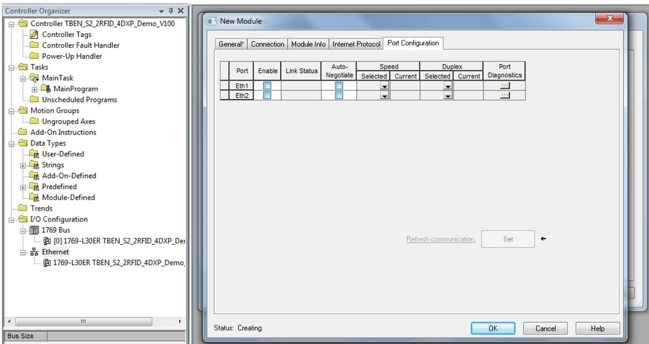
Fig. 56: Setting the port configuration
