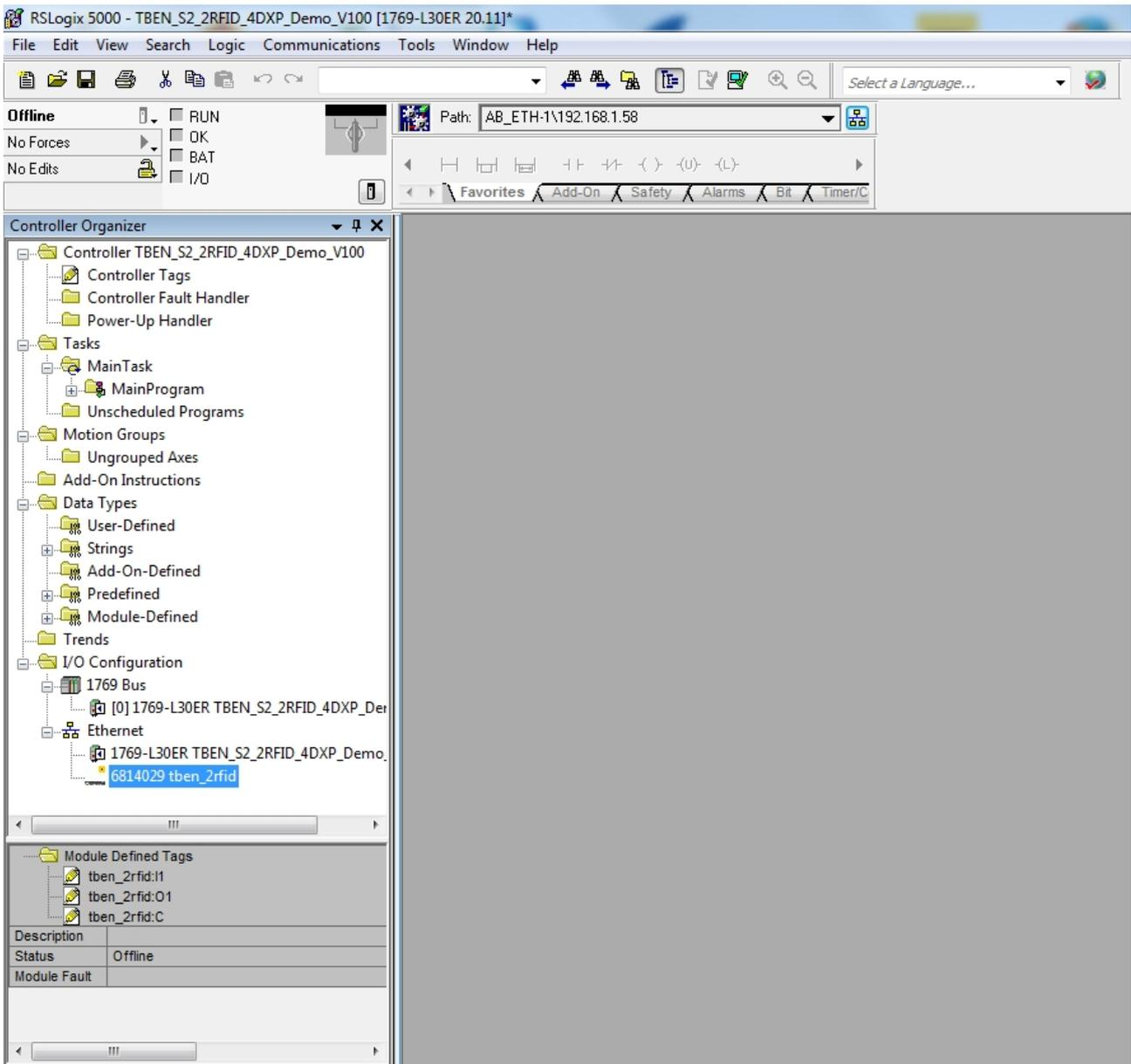
Fig. 57: TBEN-S2-2RFID-4DXP in the project tree
