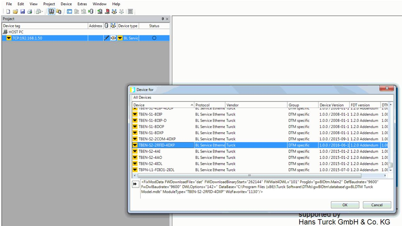
Fig. 92: Selecting TBEN-S2-2RFID-4DXP
