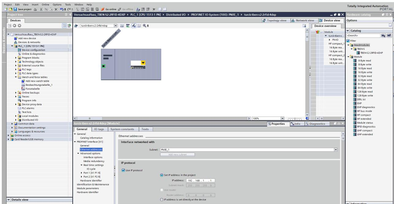
Fig. 70: Assigning the IP address
