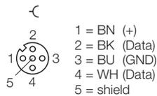
Fig. 20: .../S2500 connection cables — pin assignment of the read/write device connections
