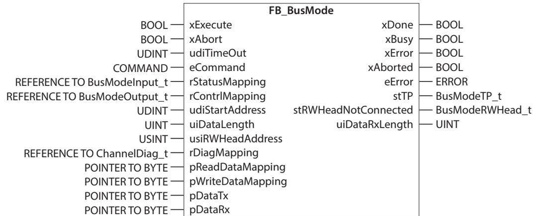
Fig. 139: FB\_BusMode function block
