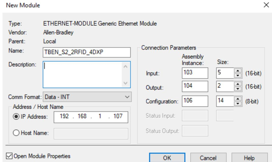
Fig. 63: Configuring the configuration assembly in RSLogix
