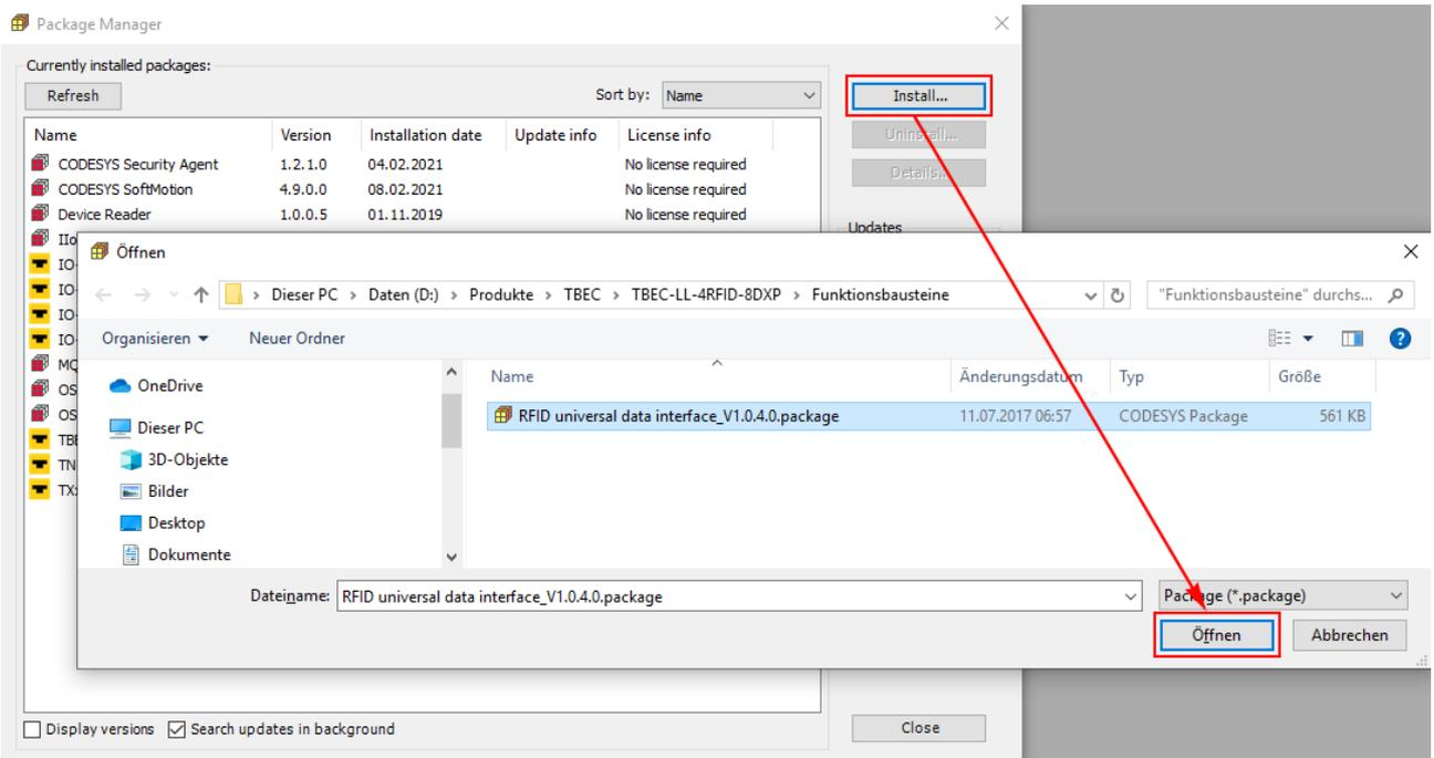
Fig. 141: Installing a Package file
