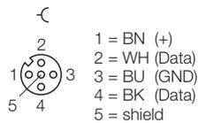
Fig. 21: .../S2501 connection cables — pin assignment of the read/write device connections
