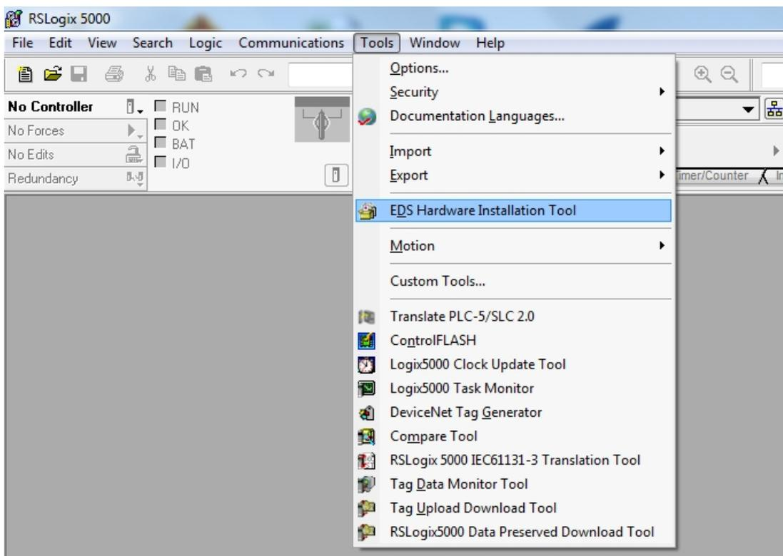
Fig. 47: Opening the EDS Hardware Installation Tool
