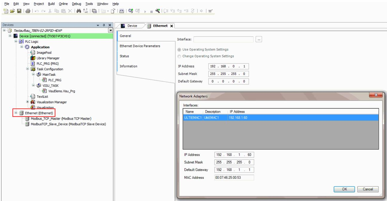
Fig. 41: Modbus master — entering the IP address (here: 192.168.1.60)
