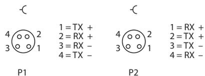
Fig. 15: Ethernet connections — pin assignment of P1 and P2
