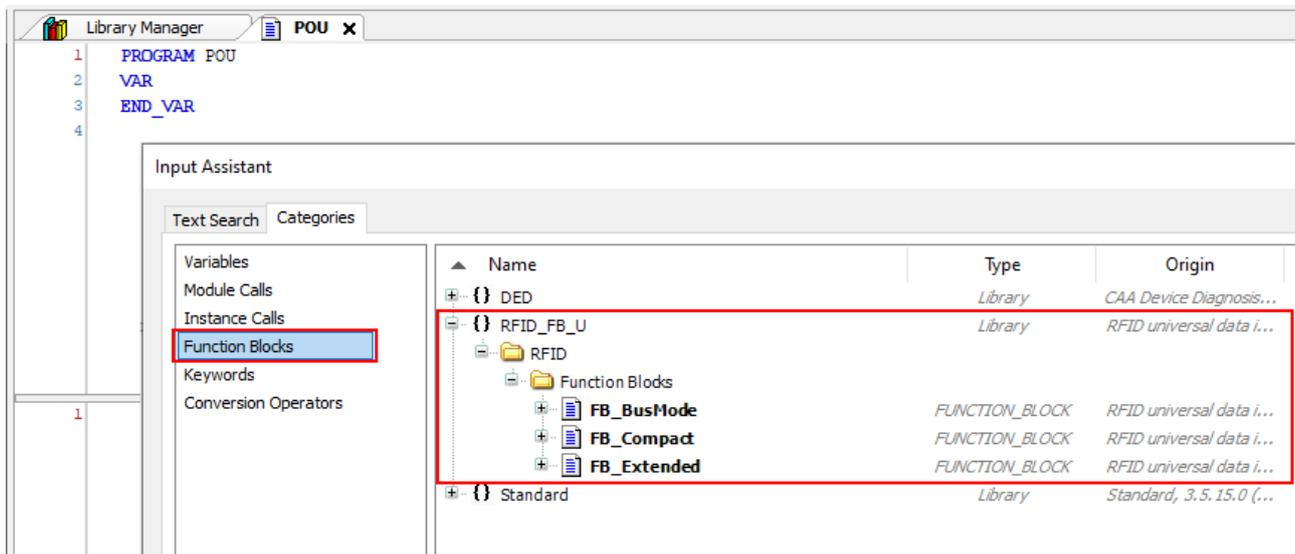
Fig. 144: Calling the CODESYS function block
