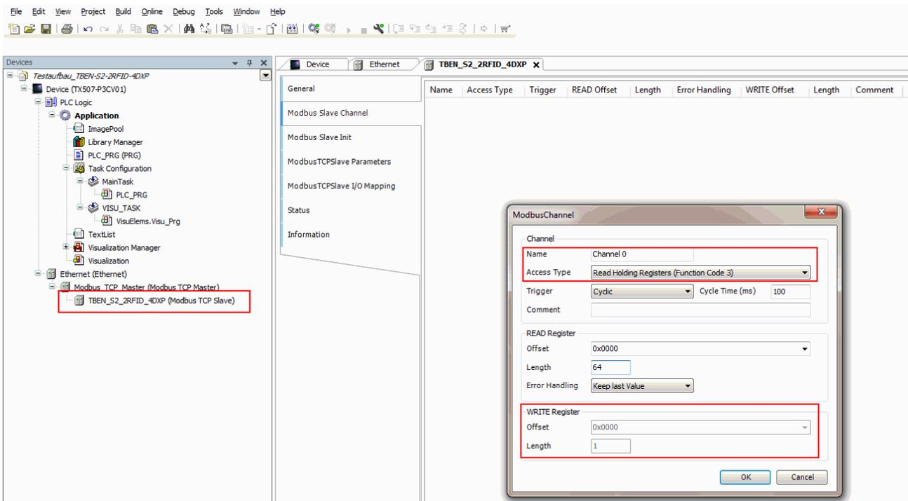
Fig. 44: Setting WRITE registers
