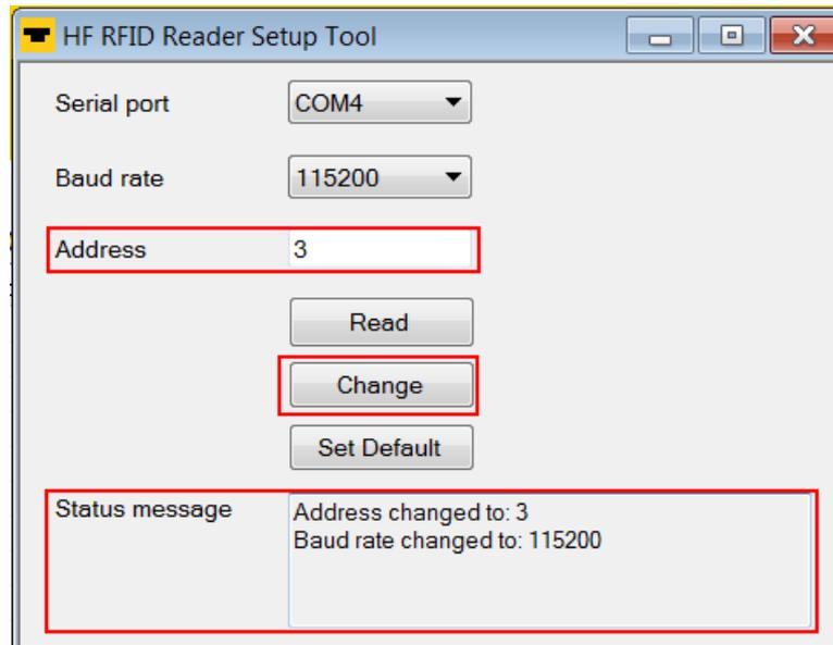
Fig. 78: Changing the read/write head address
