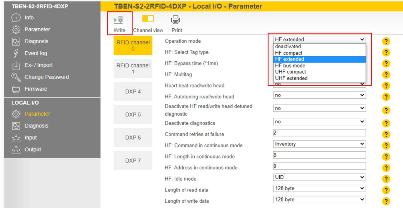
Fig. 83: Drop-down menu — operation mode
