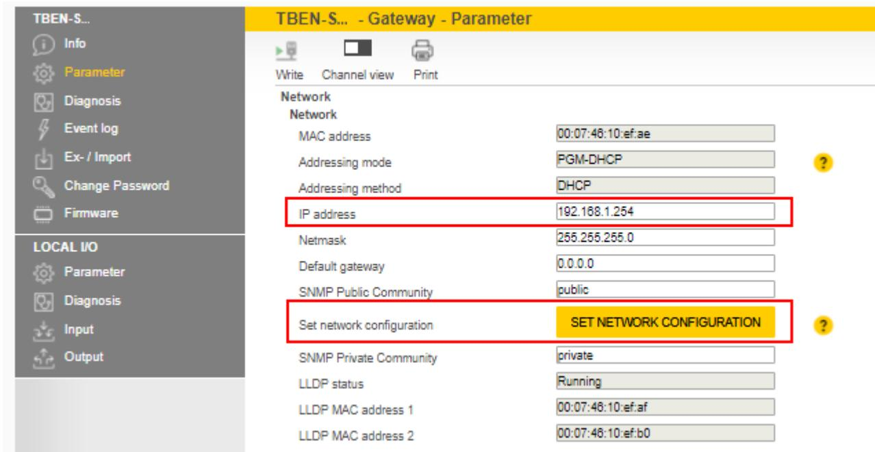
Fig. 33: Assigning the static IP address
