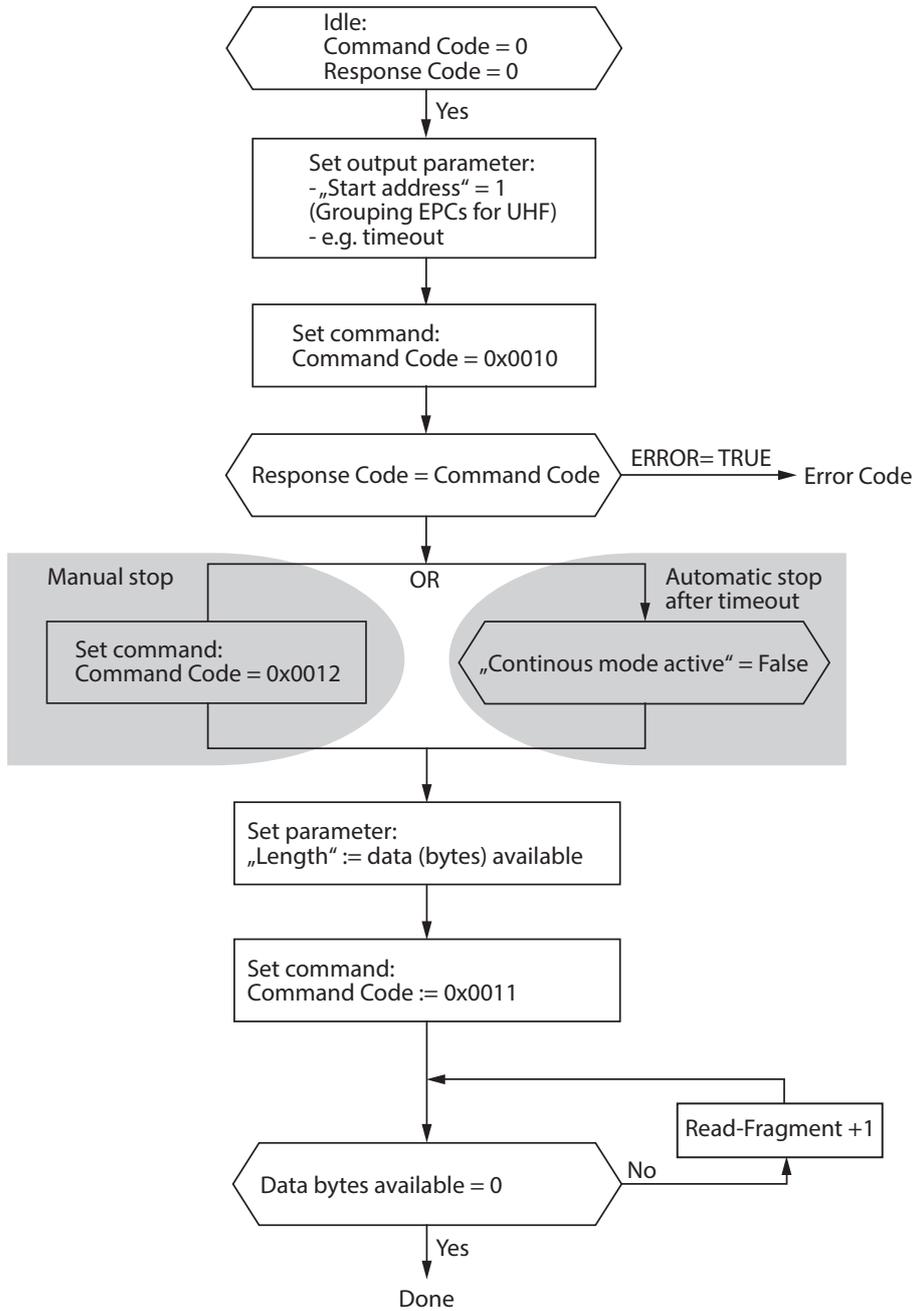
Fig. 178: Flow chart for Continuous Mode with interruption before reading data
