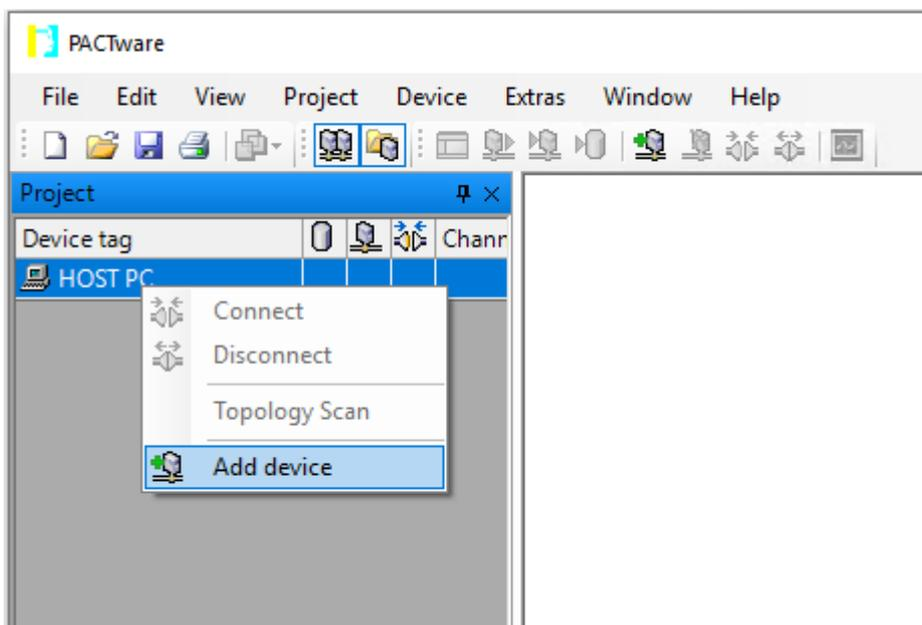
Fig. 167: Adding a device in PACTware
