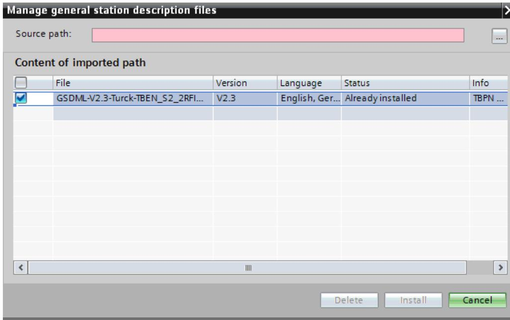
Fig. 67: Installing a GSDML file
