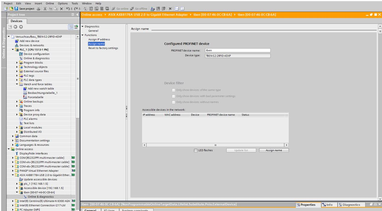
Fig. 69: Assigning the PROFINET device name
