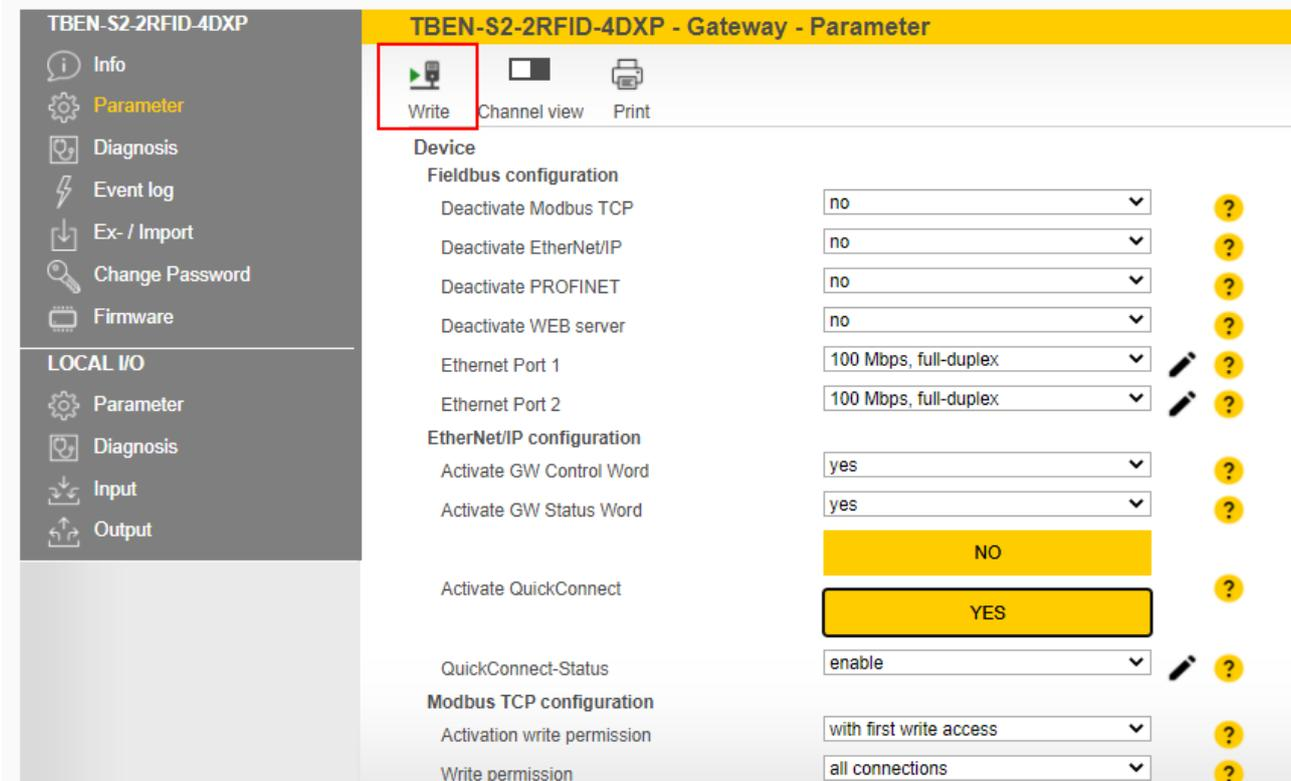
Fig. 65: Activating QuickConnect in the web server
