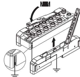
Fig. 11: Grounding the TBNN-S0-DRS... adapters
