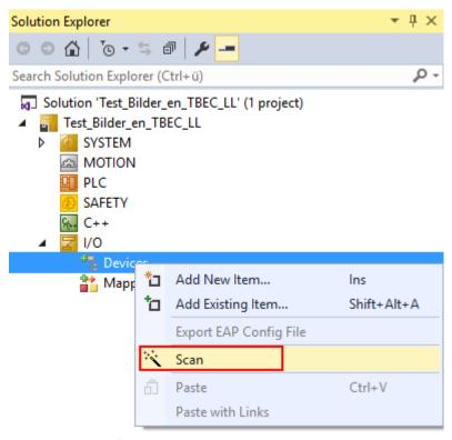
Fig. 26: Scanning for devices
