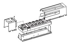
Fig. 3: Mounting the device in protection housing TB-SG-L
