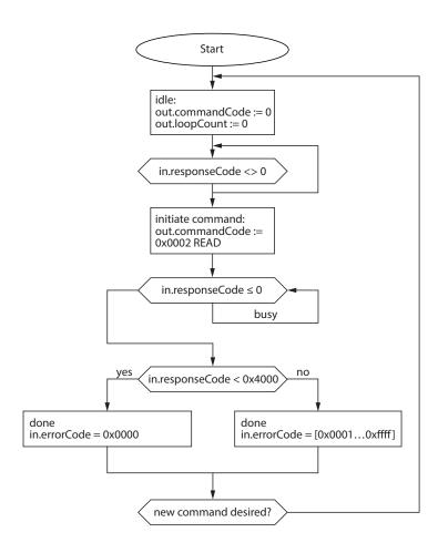
Fig. 127: Flow chart for command processing
