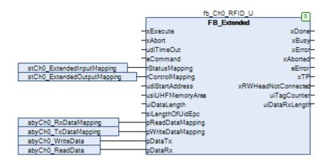
Fig. 104: FB\_Extended function block - Overview of the inputs and outputs
