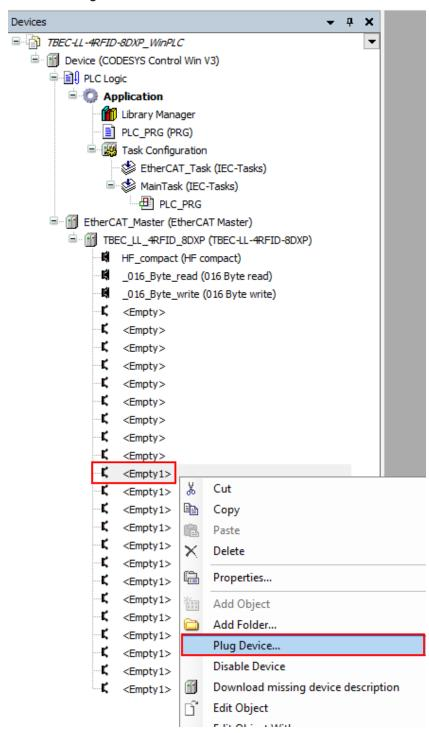
Fig. 116: CODESYS – selecting slot 13 for RFID diagnostics
