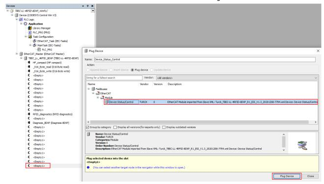
Fig. 119: CODESYS - selecting Device Status/Control
