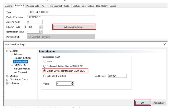
Fig. 41: TwinCAT – selecting Explicit Device Identification
