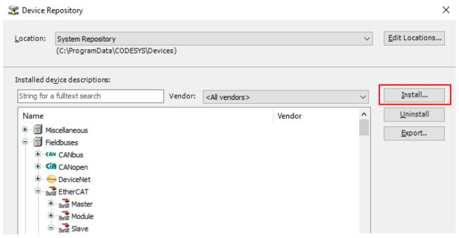
Fig. 49: Installing a device description file
