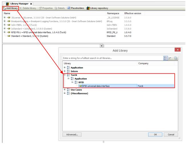
Fig. 101: Installing a CODESYS library
