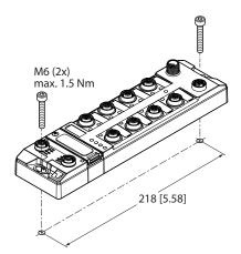
Fig. 4: Mounting the device onto a mounting plate
