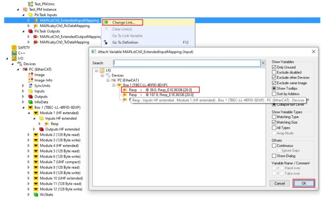
Fig. 111: Example: Linking an instance with the module register
