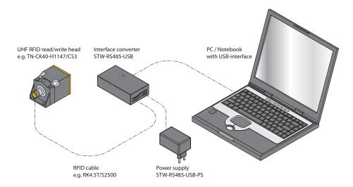
Fig. 88: Connecting the read/write head via the interface converter with a PC
