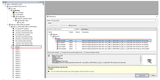
Fig. 59: Selecting HF bus mode
