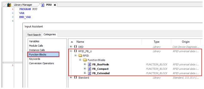
Fig. 102: Calling the CODESYS function block
