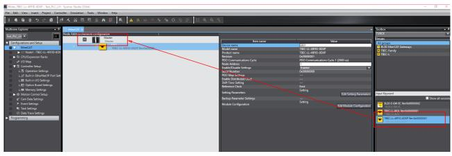
Fig. 70: Adding the device by drag and drop
