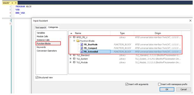
Fig. 108: Calling the TwinCAT function block
