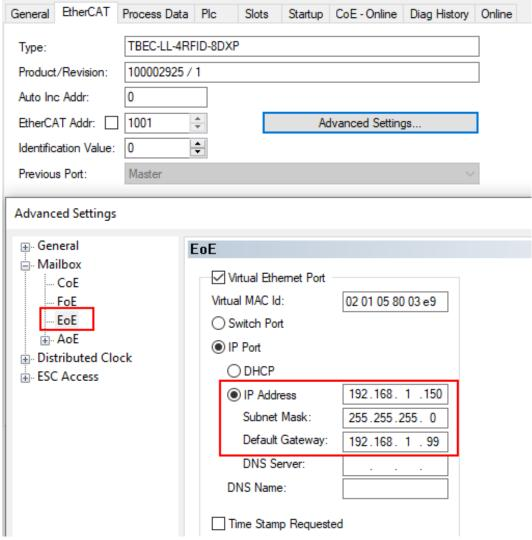
Fig. 82: TwinCAT – activating EoE in the EtherCAT slave
