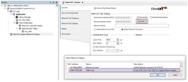
Fig. 54: Selecting a network adapter
