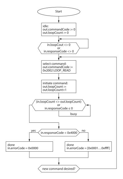
Fig. 128: Flow chart for fast command processing with loop counter
