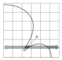
Fig. 86: Detection range of a read/write head
