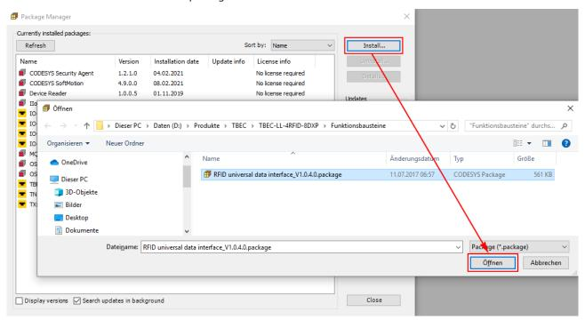
Fig. 99: Installing a Package file
