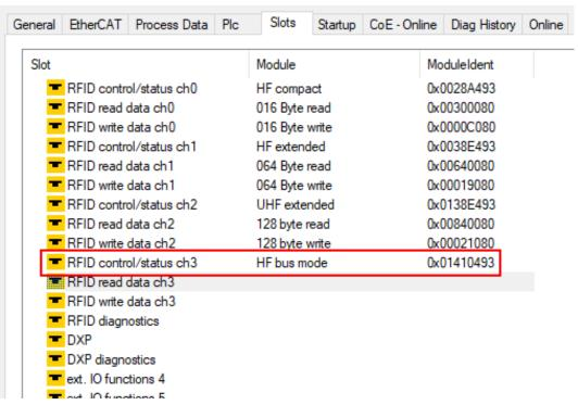
Fig. 35: HF bus mode is set for channel 3
