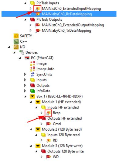
Fig. 112: Example: Successful linking between stCh0\_ExtendedInputMapping and Resp
