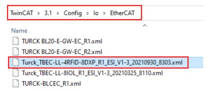
Fig. 24: TwinCAT – storing an xml file in the installation directory
