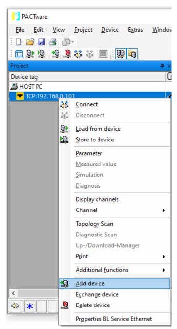
Fig. 84: DTM - Adding a device
