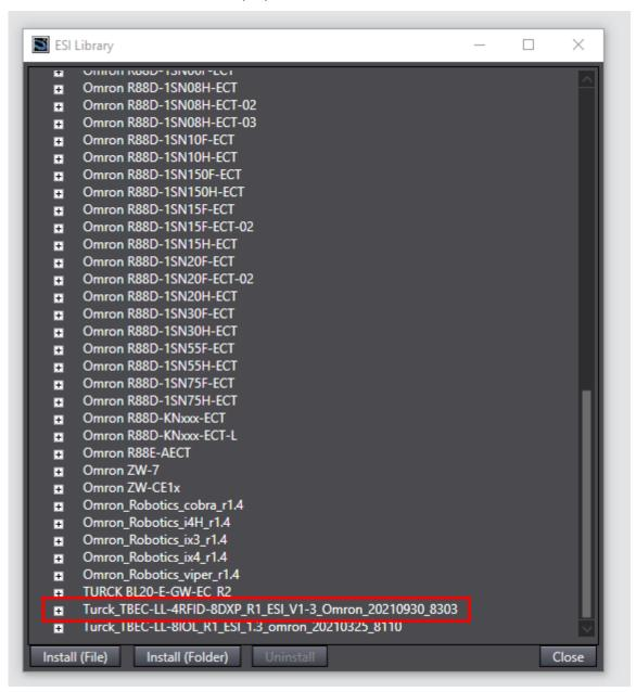
Fig. 69: Installing a ESI file
