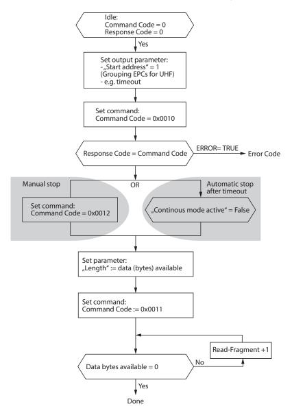
Fig. 130: Flow chart for Continuous mode with interruption before reading data
