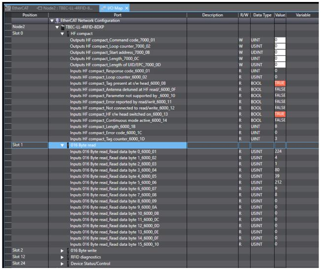
Fig. 79: I/O image of the process data in Online mode
