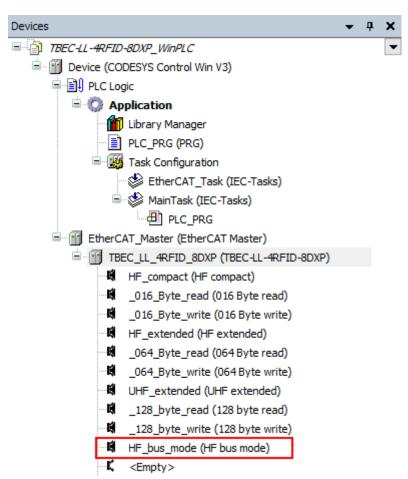
Fig. 60: HF bus mode is set for channel 3
