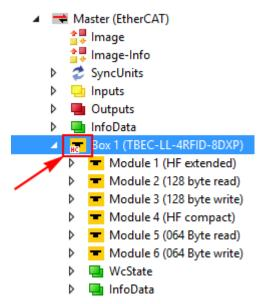
Fig. 46: TwinCAT – Hot Connect group successfully set up
