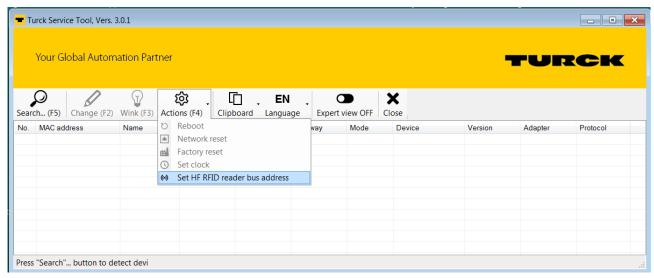
Fig. 89: Function selection – Set HF RFID reader bus address
