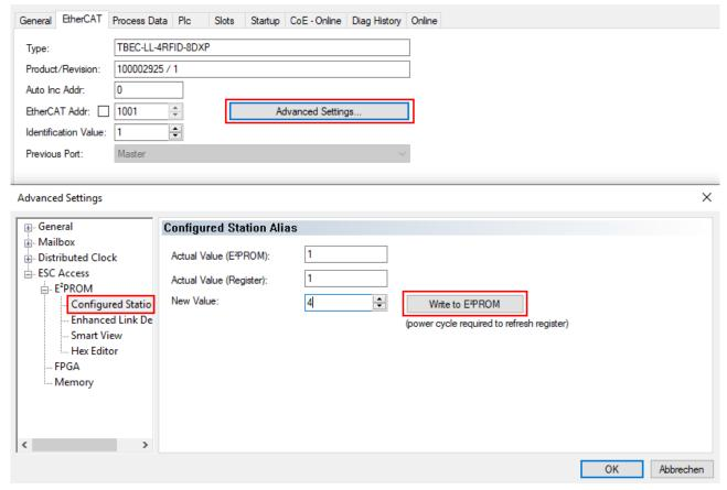
Fig. 43: TwinCAT – Configured Station Alias: entering the Identification Value
