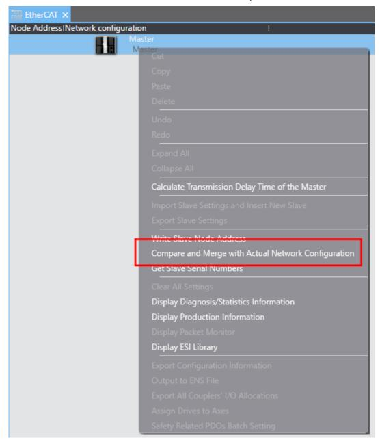
Fig. 71: Compare and merge with the actual network configuration
