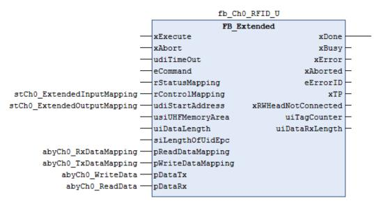
Fig. 113: Connecting an FB\_Extended function block – overview of the inputs and outputs
