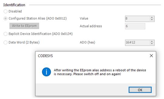
Fig. 67: CODESYS – restart required
