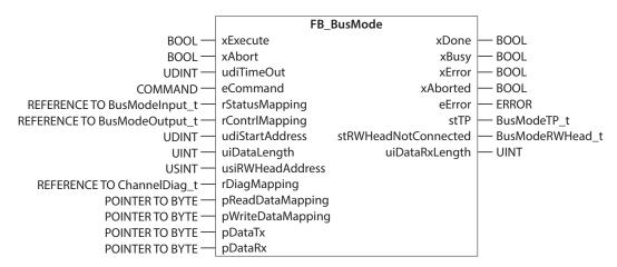
Fig. 97: FB\_BusMode function block
