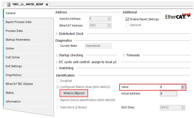
Fig. 66: CODESYS - Configured Station Alias: entering the Identification Value
