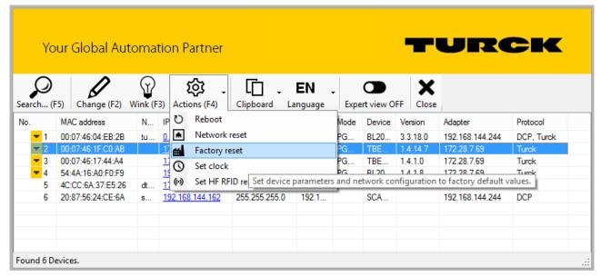
Fig. 123: Turck Service Tool – resetting the device to factory settings
