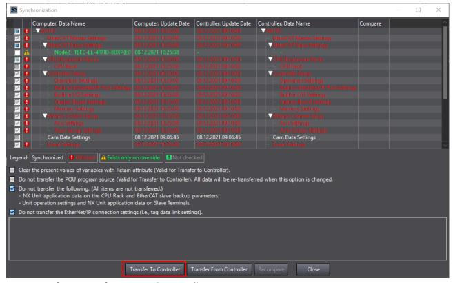
Fig. 76: Transferring a configuration to the controller
