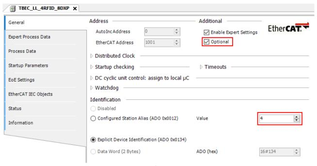
Fig. 65: CODESYS – Explicit Device ID: entering the Identification Value
