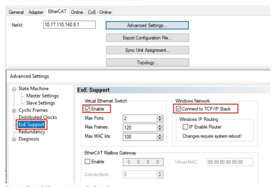
Fig. 81: TwinCAT – activating EoE in the master
