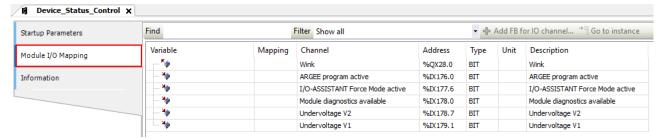
Fig. 121: Example: reading Device Status/Control
