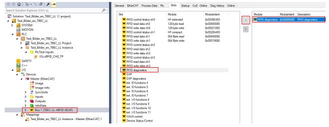
Fig. 114: TwinCAT – activating RFID diagnostics
