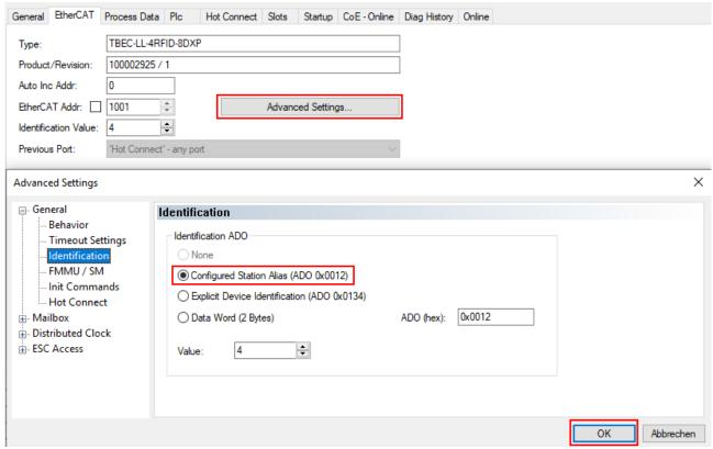
Fig. 42: TwinCAT – selecting Configured Station Alias
