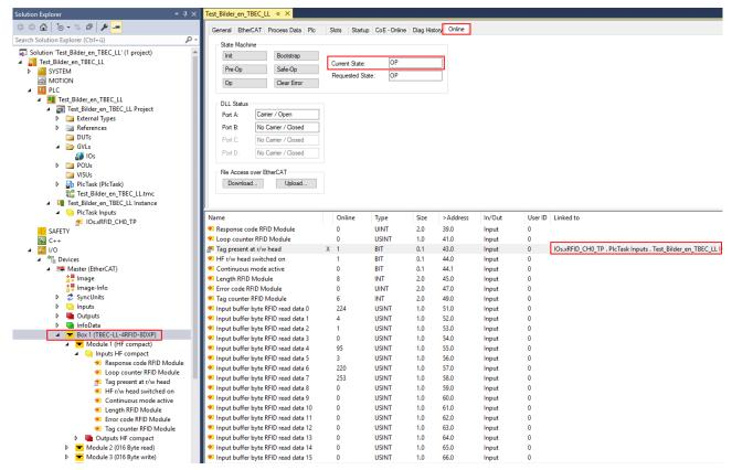
Fig. 31: EtherCAT Device – Online tab: status display (here: Operational), data points, link
