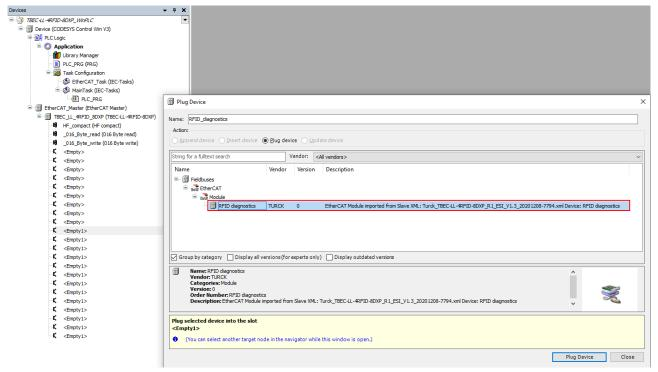
Fig. 117: CODESYS – selecting RFID diagnostics
