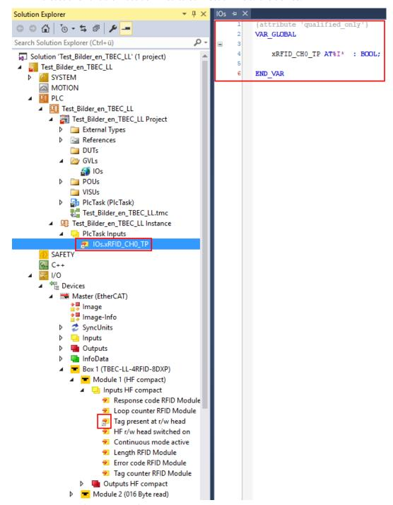
Fig. 28: Example of the linking of a variable
