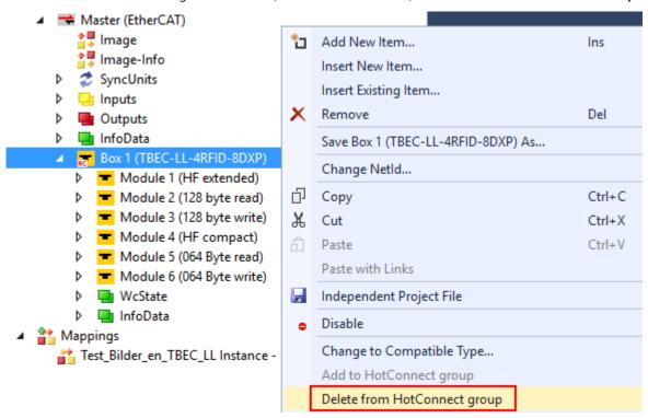
Fig. 47: Delete device from HotConnect group
