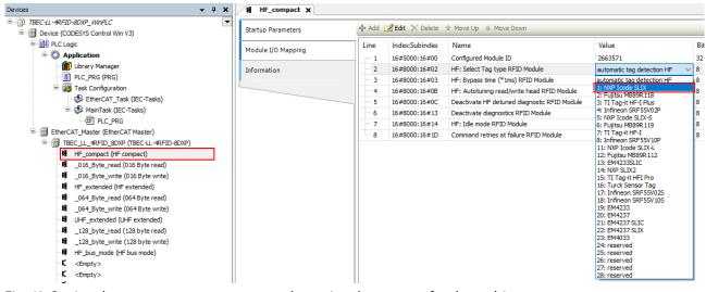
Fig. 62: Setting the startup parameters – example: setting the tag type for channel 0
