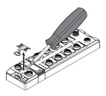
Fig. 7: Removing the grounding clamp
