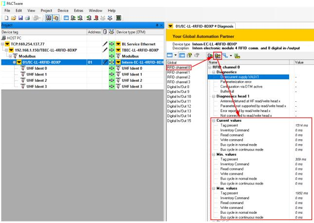
Fig. 122: Time measurement in the DTM
