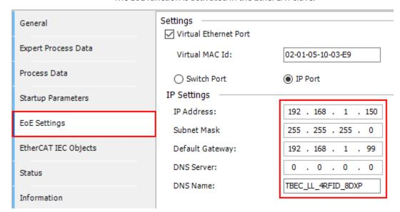
Fig. 83: CODESYS – activating EoE in the EtherCAT slave
