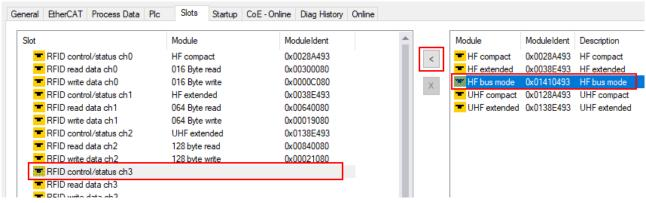
Fig. 34: Selecting HF bus mode for channel 3
