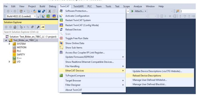
Fig. 25: TwinCAT – updating the device catalog
