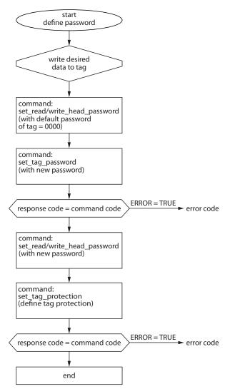
Fig. 132: Flow chart for programming tags with a password
