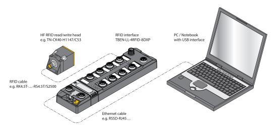
Fig. 87: Connecting read/write heads via the RFID interface with a PC
