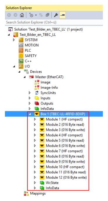
Fig. 27: EtherCAT device as Box 1 in the Solution Explorer
