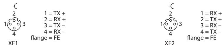
Fig. 17: Pin assignment Ethernet connectors
