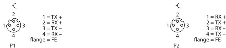
Fig. 15: Pin assignment Ethernet connectors
