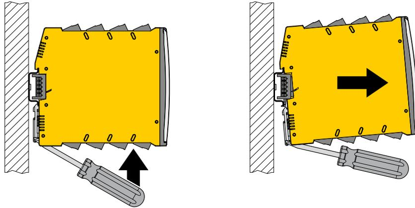
Fig. 4: Remove device
