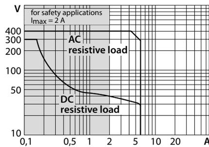
Fig. 7: Output relay load curve
