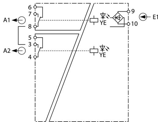
Fig. 6: Block diagram IM12-CD01-2R-1U
