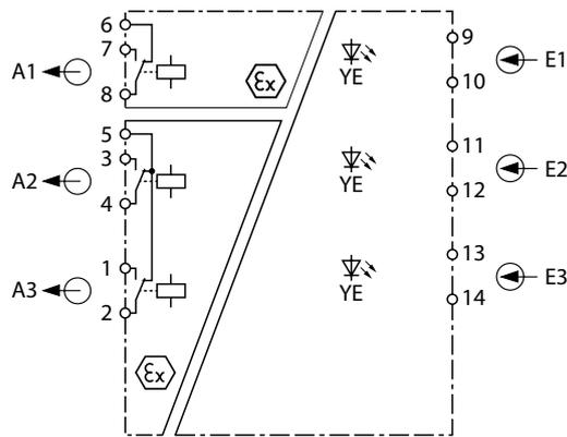
Fig. 5: Block diagram IMX12-CD01-2R-2U
